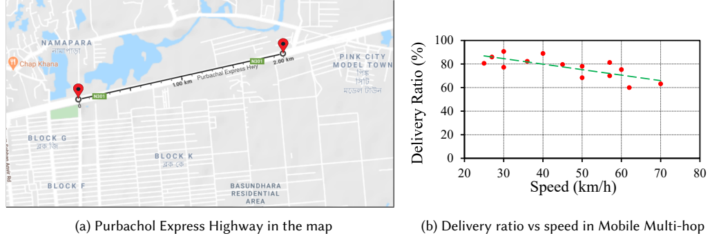
Fig. 9. LoRa Mobile Multi-hop testing from 2000m distance
